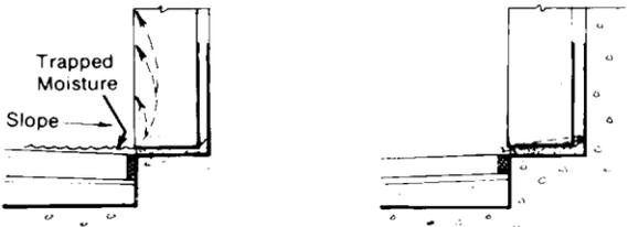
**Note:** Isolate stone from grade moisture with a concrete ledge or a dampproofed starter course with flashing as shown.
